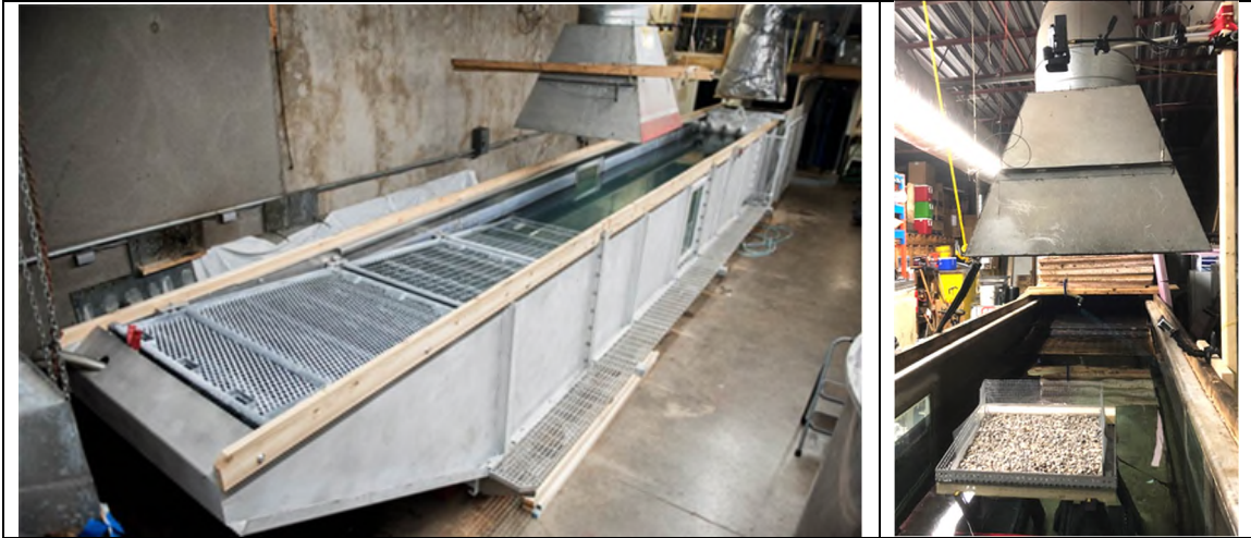
Figure 3-11: Views of Wind-Wave Tank and Test Tray mounted in the Tank
